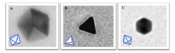
Figure 1. Representative transmission electron micrographs of the commonly observed crystalline shapes of gold nanocrystals (CNM-Au8®) resulting from our CSN® therapeutic platform. Insets are wireframes illustrating each classic shape: A, pentagonal bipyramid; B, tetrahedron; and C, hexagonal bipyramid. These nanocrystals are 10-13 nm in diameter.
